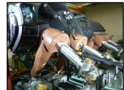
Lower limb failure evaluation test facilities
