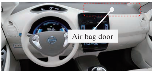
Fig. 1 Air bag door on the Nissan Leaf instrument panel
